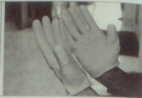
Fig. TC. 10. Handgloves produced from room temperature vulcanization.
