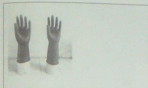
Fig. TC. 6. General purpose gloves prepared from blends of NR/XSBR 80:20
