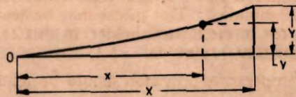
FIG. 8 PRINCIPLE OF REBOUND RESILIENCE MEASUREMENT
