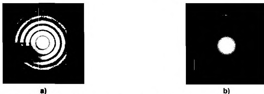
Figure 1 — Scattering pattern for two spherical particles: the particle generating pattern a) is twice as large as the one generating pattern b) (simulated images for clarity)
