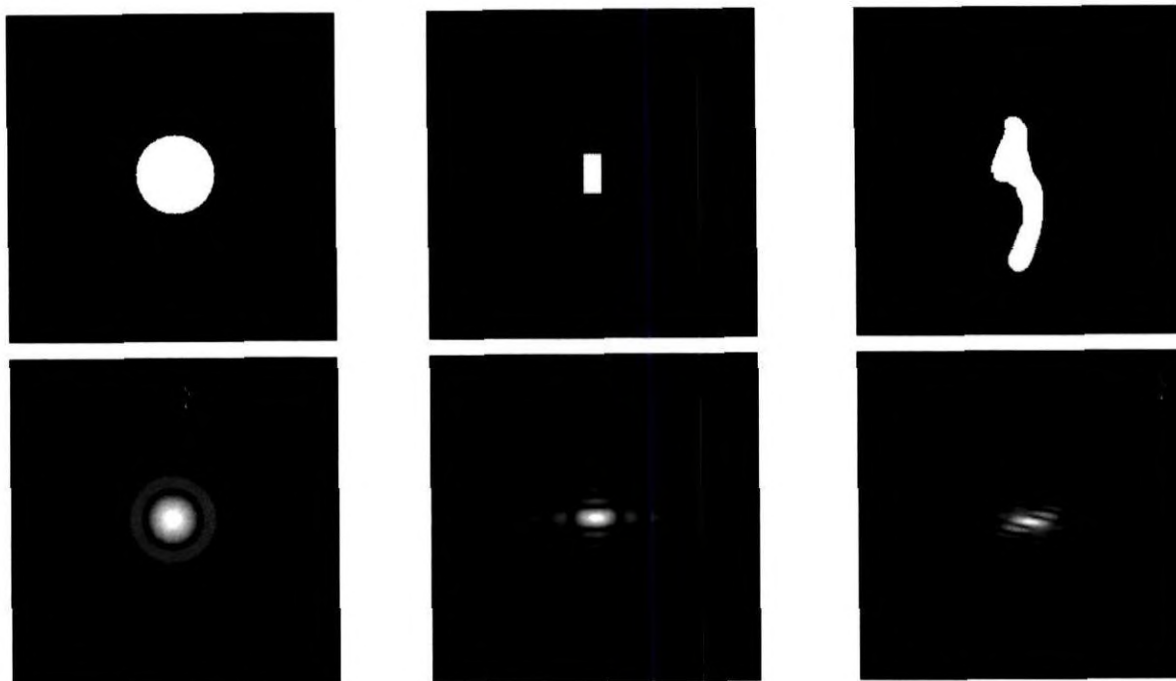
Figure A.12 — Circular, rectangular and irregular particles and their scattering patterns (simulated images)
