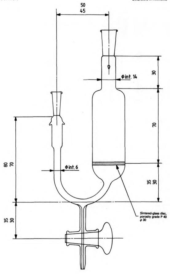
Figure 2 - Absorption vessel for use in the determination of total sulfur by the furnace combustion method
