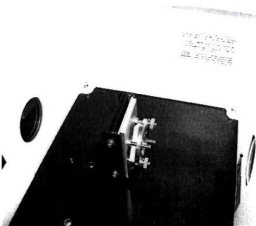
Figure A.7 — Plate holder mounted in the IR spectrometer
