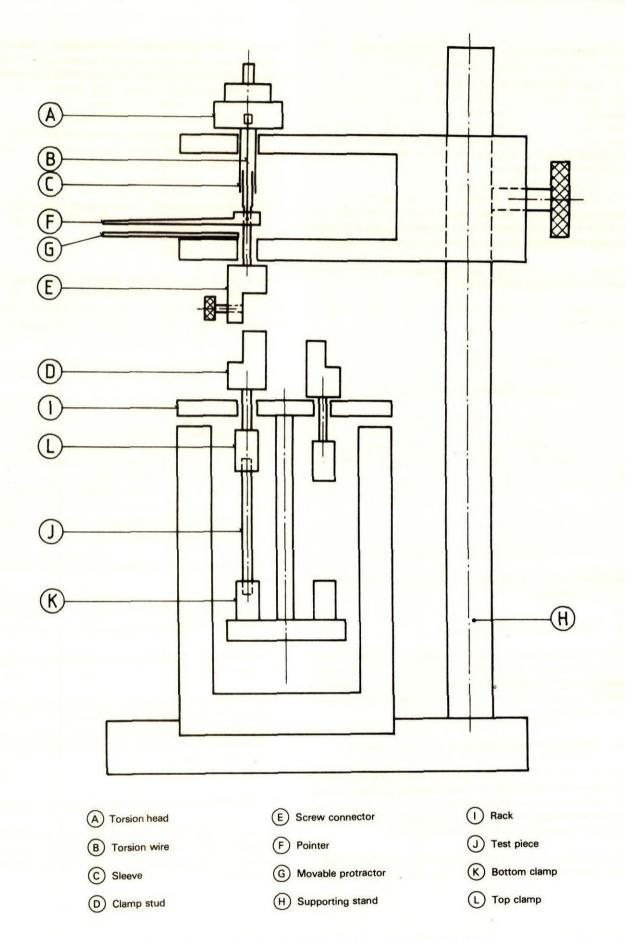
Figure — Apparatus for determination of stiffness characteristics
