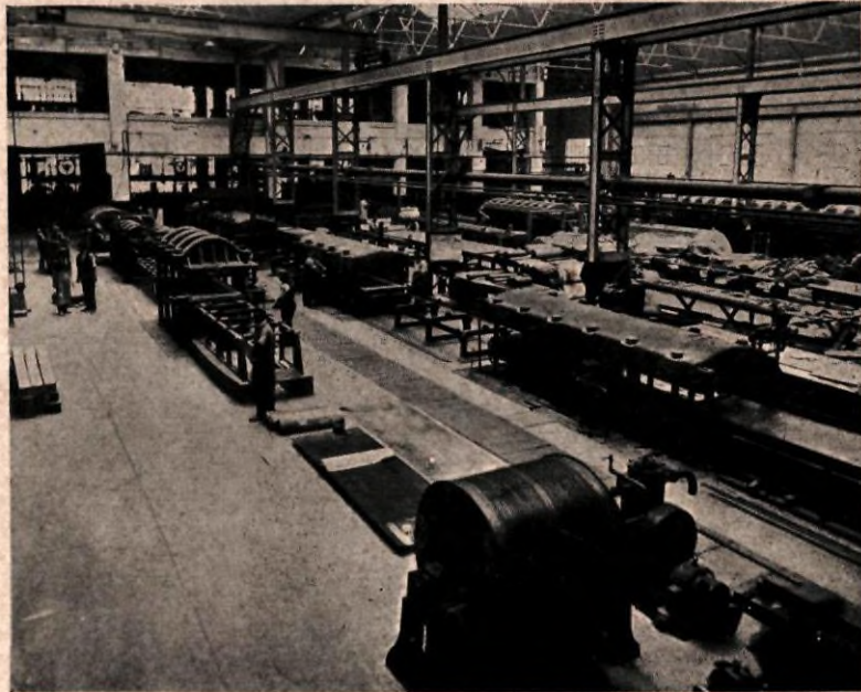
GENERAL VIEW OF RUBBER FACTORY SHOWING VULCANISING PRESSES USED IN THE MANUFACTURE OF RUBBER FLOORING
