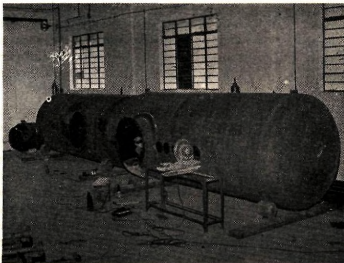
Photograph showing Rubber-lining of tank in process.
