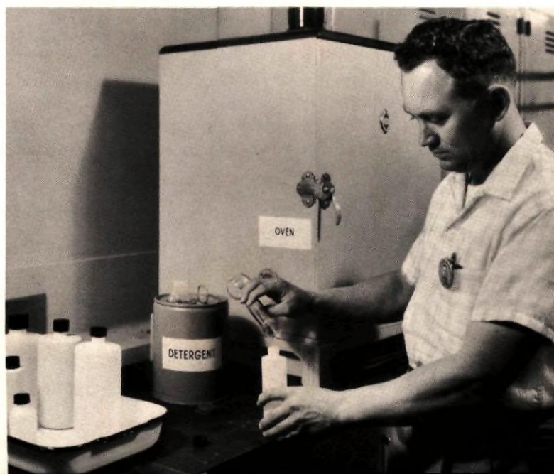
Preparing samples for accelerated aging at high temperatures.
