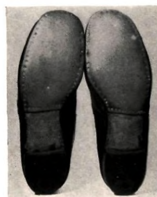
Riveted half sole
