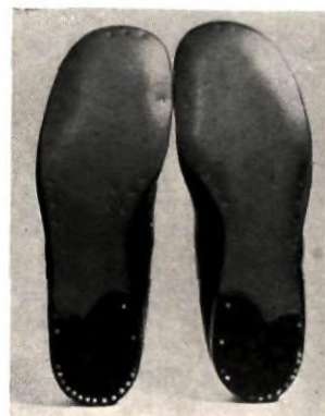
Stuck-on through sole
