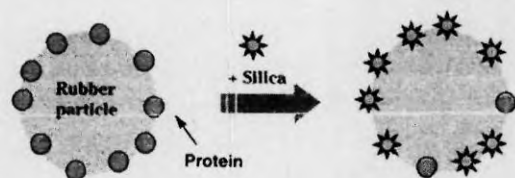
Figure 3. Replacement of rubber bound proteins by silica
