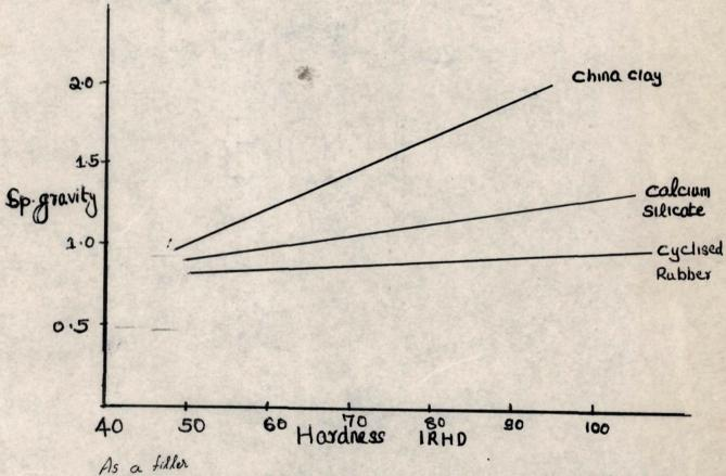
Acyclised rubber is superior to calicum silicate and precipitated calcium carbonate but slightly inferior to aluminiam silicate, when the physical properties such as harmess hardness and tensile strength are compared as shown in the following charts.
