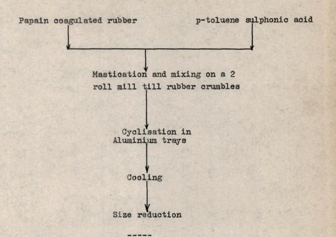
Excess axid acid present in the product has to be neutralised. Products used in reinforcing application is neutralised by incorporating calcium oxide. In the case of solution applications, the excess acid is removed by washing first with water followed by ammonium hydroxide or sodium carbonate and then finally with water.
