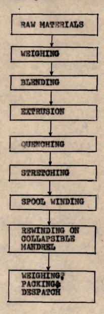
Plastic cames are produced by the extrusion process.
