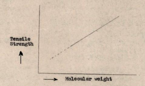
The tensile strength increases as molecular weight increases with in a practical range of somewhat below 100,000 to about 400,000.
