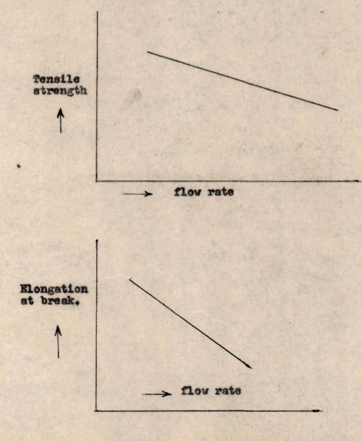
The flow rate through the die is thus an important parameter affecting the tensile properties of the extruded cane.
