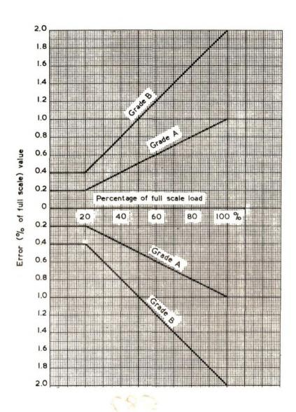
Figure 1. Machine accuracy gradings from BS 1610:
