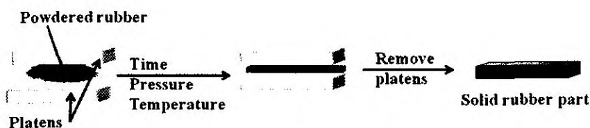
Fig. 17. General representation of the process of high pressure high temperature sintering
