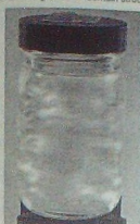
Figure 2: 0.02% dispersion of Microbe ® in water showing oriented domain structure.
