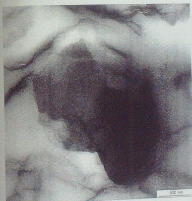
Figure 2. TEM images taken at various magnifications from the film cast of PUR latex containing 10phr LS
