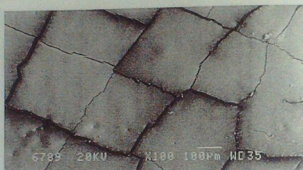
Figure 16. SEM micrograph of UV-15 cm-2 min treated vulcanised latex 2.
