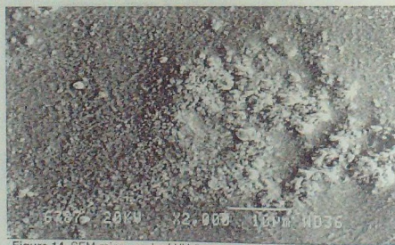
Figure 14. SEM micrograph of UV-5 cm-5 min treated vulcanised latex 1.
