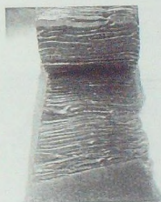
Figure 8. Photograph showing the cohesive failure in 3 wt% TCI-EA treated latex 2/PU adhesive + polyisocyanate/leather joints.
