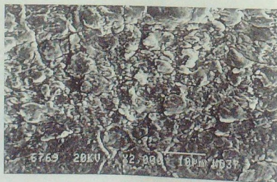
Figure 2. SEM micrograph of as-received vulcanised latex 1.
