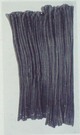
PLATE J. Twenty pairs of socks returned after a wearing trial; those in the top pile were given a chemical treatment, those in the lower a rubber finish.
