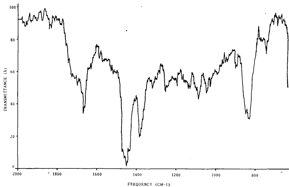
Fig. 4. IR spectrum of depolymerized rubber
