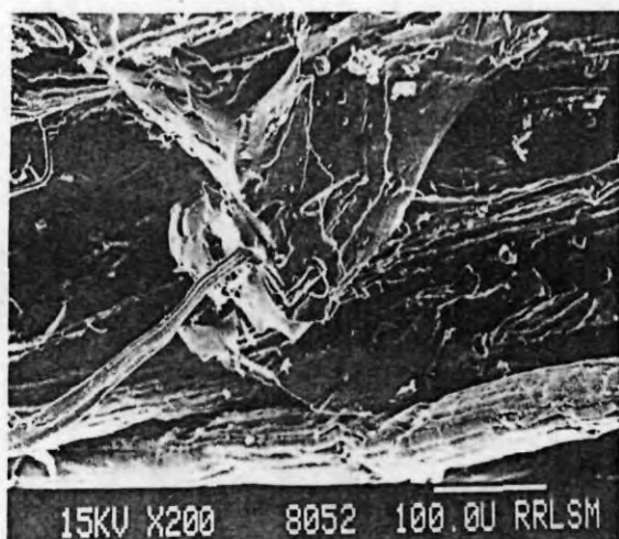
Figure 12 SEM photograph showing better adhesion between fiber and matrix on transverse orientation.
