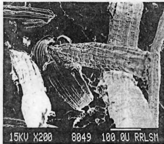
Figure 11 SEM photograph showing better adhesion between fiber and matrix in longitudinally oriented composite containing bonding agent (mix L).
