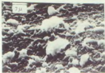
Fig. 21 SEM photomicrograph of blend C 6 (70 NR-30 HDPE-40 HAF) extruded at a shear rate of 1223 s -1 .
