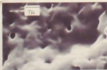
Fig. 17 SEM photomicrograph of blend C (70 NR-30 HDPE) extruded at a shear rate of 122 \text{ s}^{-1} . Figure shows a region close to the axial surface of the extrudate.
