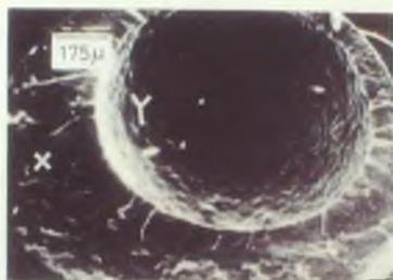
Fig. 12 SEM photomicrograph of blend B (50 NR-50 HDPE) extruded at a shear rate of 122 \text{ s}^{-1} .
