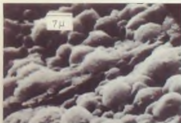
Fig. 15 SEM photomicrograph of blend C (70 NR-30 HDPE) extruded at a shear rate of 12 \text{ s}^{-1} .
