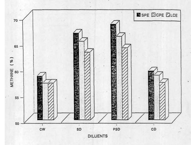
Fig 3 Methane content in the biogas with different diluents.
