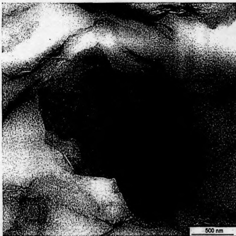
Figure 2. TEM images taken at various magnifications from the film cast of PUR latex containing 10phr LS
