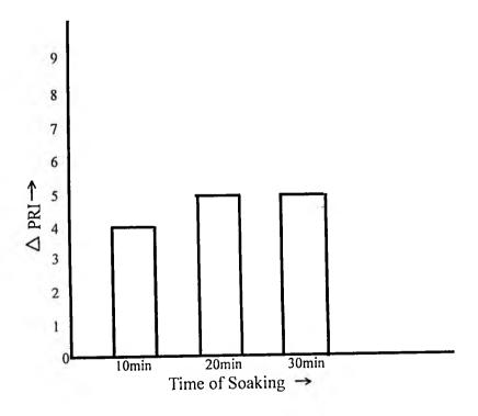
when crumbs of raw natural rubber are soaked in a solution of oxalic acid, for imparting protection to rubber oxalic acid has to enter into rubber. Entry of oxalic acid is via a diffusion mechanism since this a time controlled process, the optimum duration of soaking had to be decided. For this crumbs were soaked in 0.1% oxalic acid solution for varying duration and PRI of rubber were determined. The results obtained are shown in figure.
