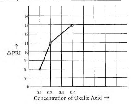
The results obtained are shown in figure. From the graphs it is clear that, on increasing the concentration of oxalic acid from 0.1% onwards PRI of rubber sample increases; however the increase is only nominal over 0.1%. Hence it was concluded that oxalic acid concentration of 0.1% was the optimum. Further studies were conducted at 0.1% concentration.
