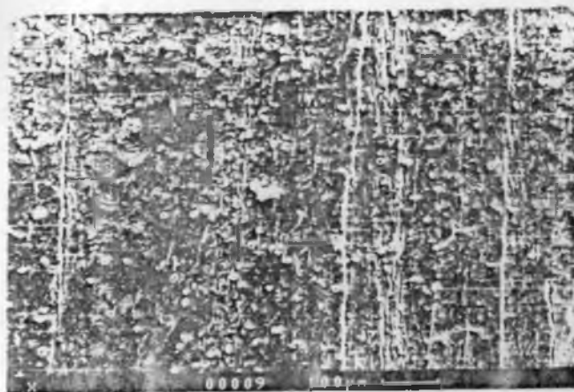
Fig. 3.2.15: Abraded surface of gum XNBR vulcanizate showing clear surface.
