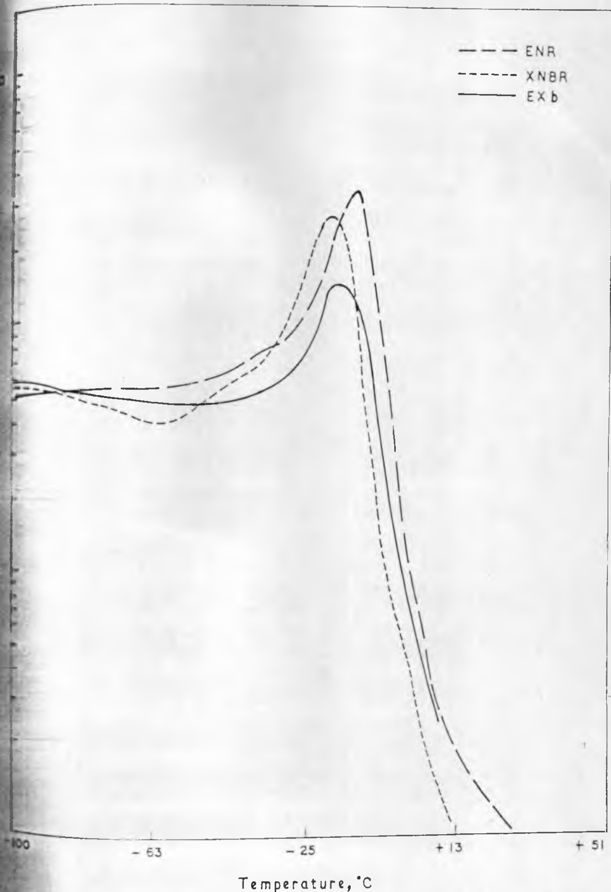
Fig. 3.3.2 : Plots of viscous modulus versus temperature for ENR, XNBR and the 1:1 ENR-XNBR blend vulcanisates.
