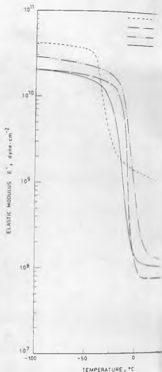
Figure 6 Elastic modulus ( E' ) plots of Neoprene, ENR, XNBR and the ternary blend
