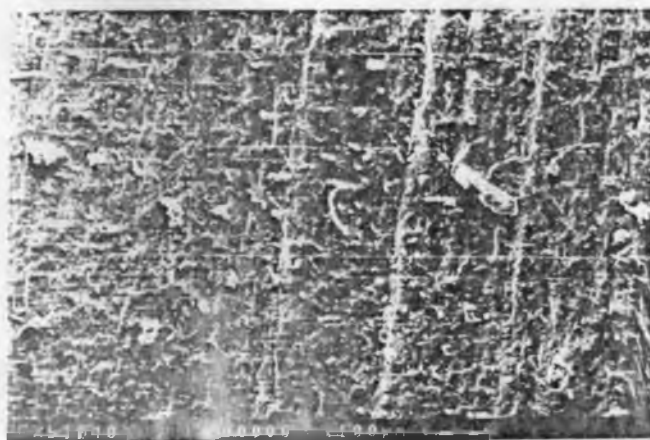
Fig.3.2.19 : Abraded surface of 1:1 ENR-XNBR blend filled with 40 phr ISAF black showing closely packed fine ridges.
