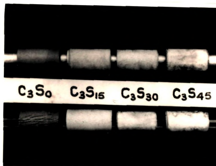
Figure VI.A.9 Photograph of blend C (80:20 NR:EVA) having different silica content after 8 h and 85 h of exposure to ozonised air.
