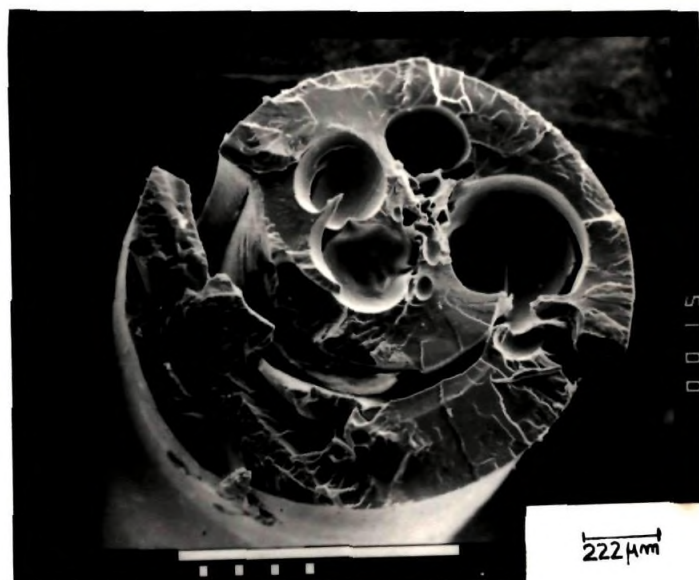
Figure V.13 SEM Photomicrograph of blend H extruder at a shear rate of 330 s -1 .
