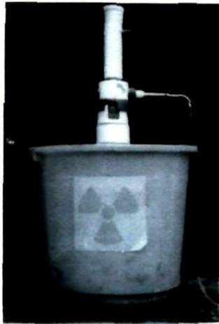
Plate 7 Field dispenser for ^{32}\text{P} application
