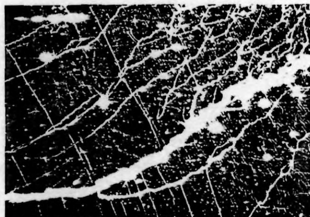
FIG. III.24 : Tensile fracture of sulfur-cured unfilled SBR; smooth surface with tear lines.
