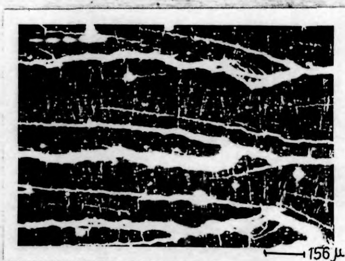
FIG. III.8 : Tear fracture of sulfur-cured unfilled NR; branching of tear lines.
