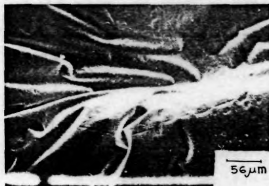
Figure 5 V-shaped foldings in the tear zone of the opened-up craze in tensile failure of 1,2 PB.
