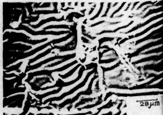
Figure 8 Foldings, lips and fibrils on the tensile failure surface of K1107.
