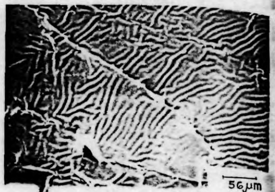
Figure 7 Smooth fracture path with foldings in tensile failure of K1107.
