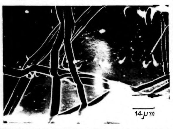
FIG.VII.B.5 NETWORK OF CHANNELS INSIDE THE CENTRAL STRESS ZONE IN TENSILE FAILURE OF PB
