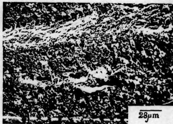
FIG.IV.D.6 TEAR FRACTOGRAPH OF BLEND DS; BROAD CONTINUOUS TEAR PATH
