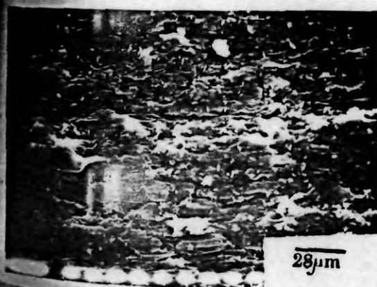
FIG.IV.E.8 SEM PHOTOGRAPH OF ABRADED SURFACE OF BLEND DS; SHALLOW GROOVES
