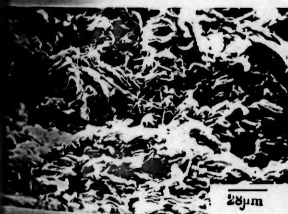
FIG. IV.D.3 TEAR FRACTOGRAPH OF BLEND DU; SMOOTH TEAR PATH AND ROUGH SURFACE
