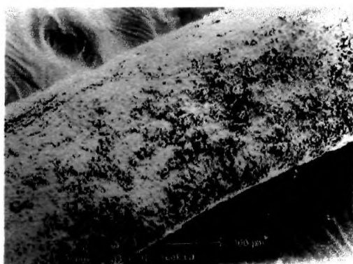
Figure 3.10 SEM of isocyanate treated OPEFB fibre surface (x100)
