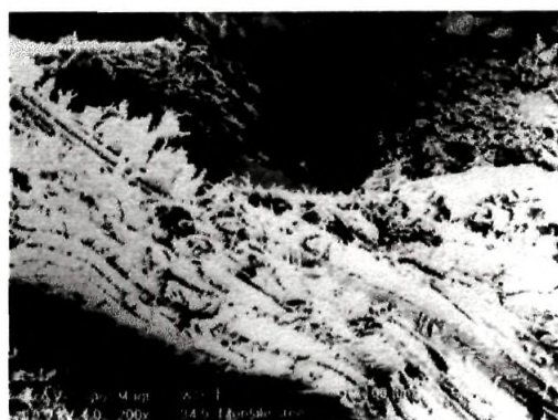
Figure 4.8 SEM of tensile fracture of KMnO 4 oil palm fibre/PF composite(x200)
