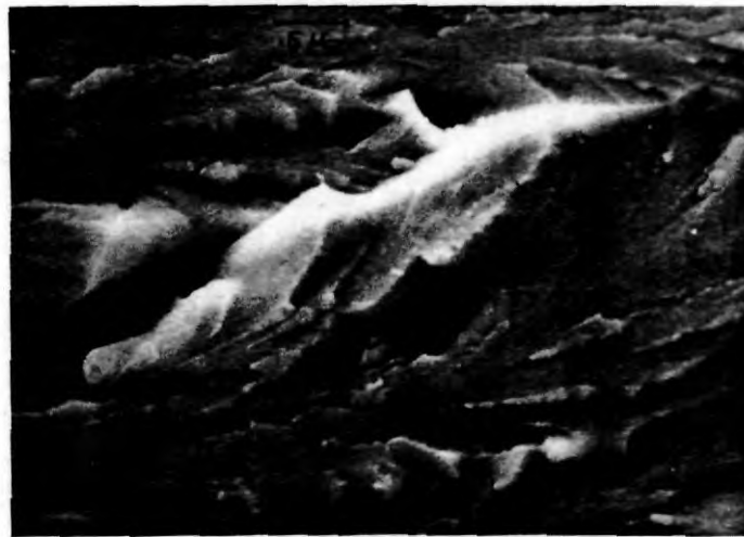
Fig. 9: Scanning electron micrograph of tensile fracture surface of neat phenol-formaldehyde sample (x 800).
