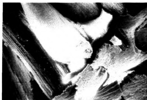
Figure 4.17 SEM of impact fracture of silane treated oil palm fibre/PF composite (x100)
