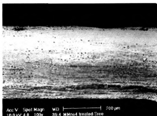
Figure 3.8 SEM of permanganate treated OPEFB fibre surface (x100)
