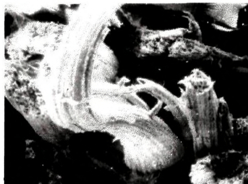
Figure 4.5 SEM of tensile fracture of alkali treated oil palm fibre/PF composite (x100)
