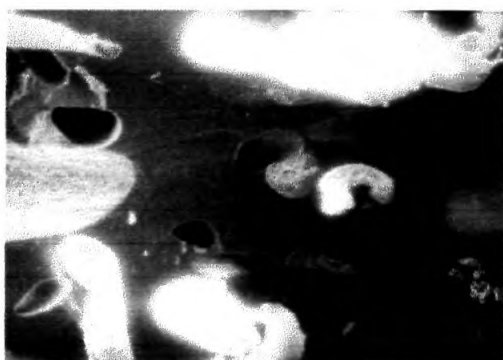
Figure 4.15 SEM of impact fracture of acetylated oil palm fibre/PF composite(x50)
