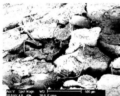
Figure 9.21 SEM of impact fracture of gamma irradiated, silane treated oil palm fibre/PF composite.(x49)
