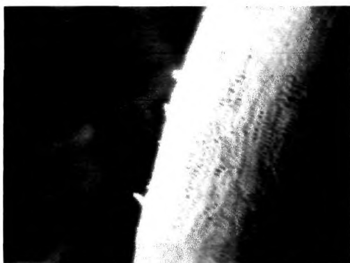
Figure 3.6 SEM of acetylated OPEFB fibre surface (x200)
