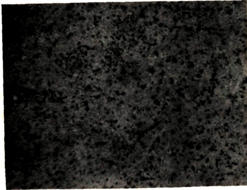
Fig. 4.10. Optical micrograph of PVL film containing 5 phr of silica (x 120)
