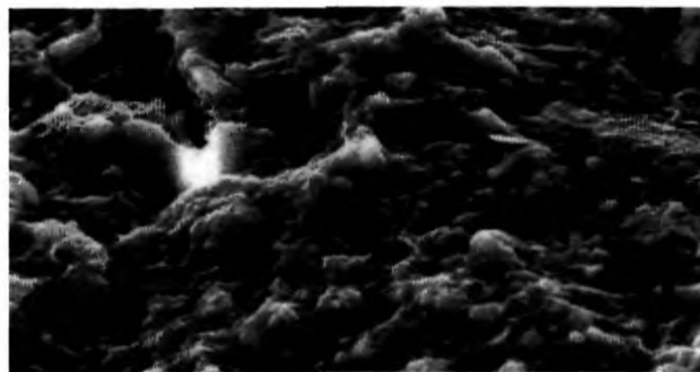
Figure 1. 5 Scanning electron micrograph of montmorillonite. Divided platy forms with poorly defined shapes and very crumpled layers
