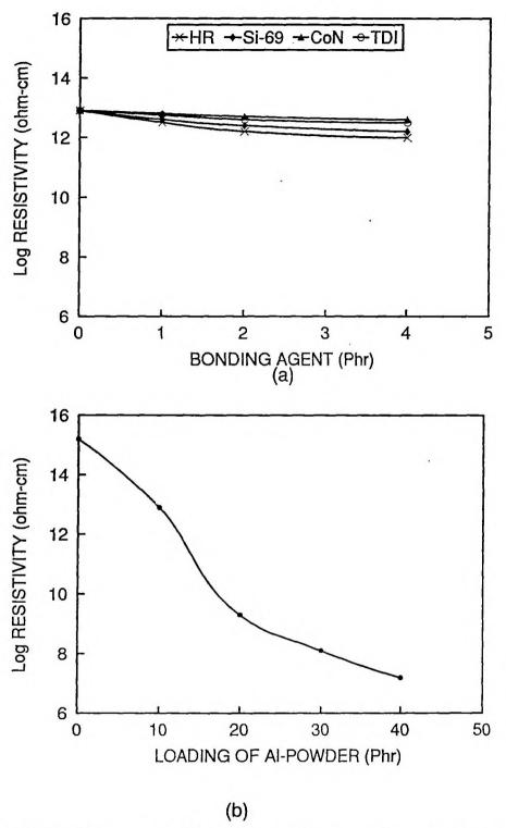
Figure III.10. Volume resistivity of NR-aluminium powder composites as a function of (a) the amount of bonding agent and (b) the amount of aluminium powder without bonding agent
