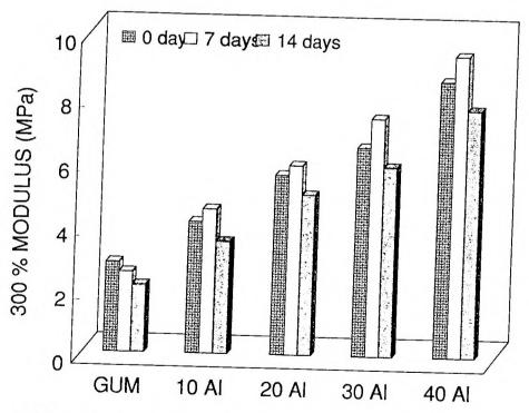
Figure VIII.3. Variation of modulus (300%) of aluminium powder filled natural rubber composites after ageing at 70°C
