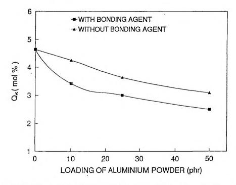
Figure IV.5. Effect of aluminium powder on equilibrium sorption (swelling solvent — toluene at 27°C)
