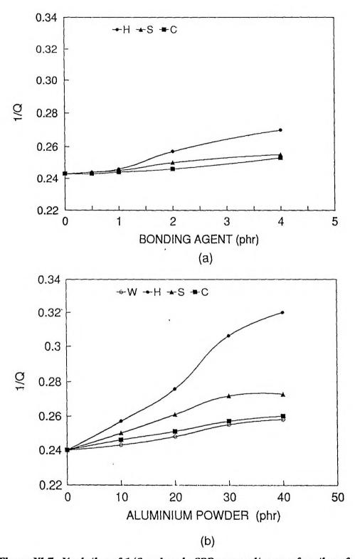
Figure XI.7. Variation of 1/Q values in SBR composites as a function of (a) the amount of bonding agent at 10 phr of aluminium powder (b) the amount of aluminium powder
