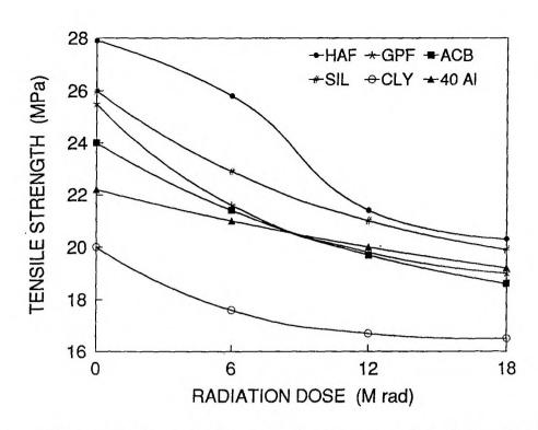
Figure VIII.6. Variation in tensile strength with gamma irradiation for NR-vulcanizates containing different fillers
