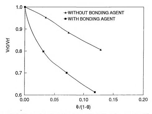
Figure IV.8. Kraus plots of swelling data. Effect of bonding agent on NR-aluminium powder composites
