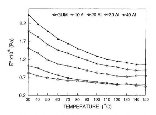
Figure VII.5. Dependence of E" with temperature of aluminium powder filled natural rubber composites at a frequency of 10 Hz
