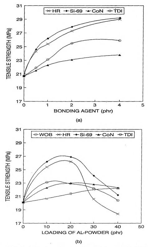
Figure III.4. Variation in tensile strength values as a function of (a) the amount of bonding agents on natural rubber-aluminium powder (10phr) composites and (b) the amount of aluminium powder in NR
