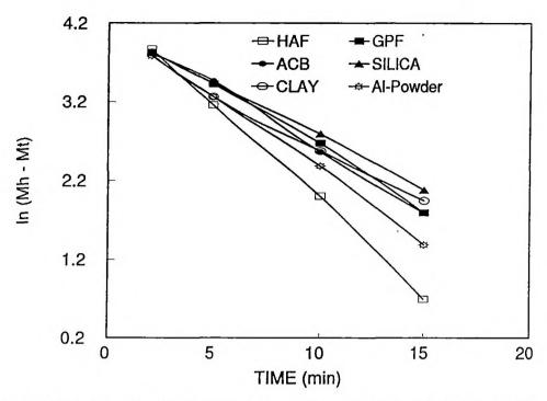
Figure V.1. Kinetic plot for the cure reaction of various filler (40 phr) incorporated natural rubber composites
