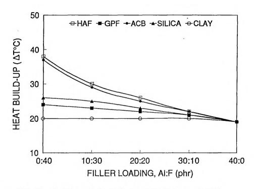
Figure V.6. Heat build-up of aluminium powder incorporated NRcomposites in presence of various fillers
