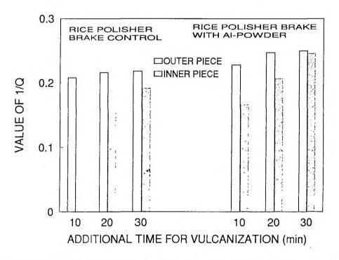
Figure IX.4 1/Q values of inner and outer pieces of 5 cm cube of rice polisher brake compound with and without aluminium powder
