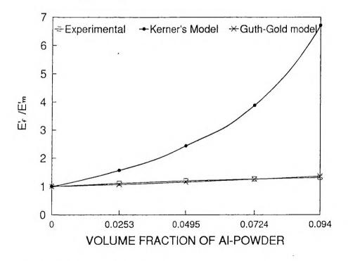
Figure VII.15. Relative modulus E'./E'... as a function of aluminium powder concentration at 35°C, 10 Hz
