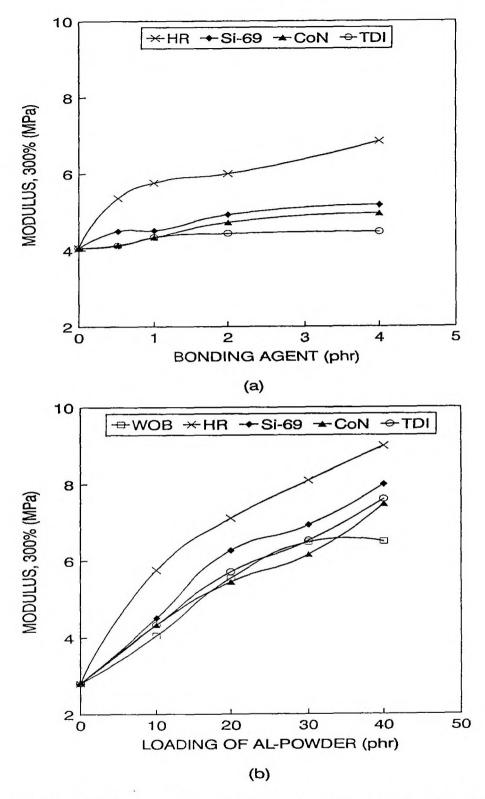
Figure III.3. Variation in modulus at 300 % elongation as a function of (a) the amount of bonding agents on natural rubber-aluminium powder (10 phr) composites and (b) the amount of aluminium powder in NR
