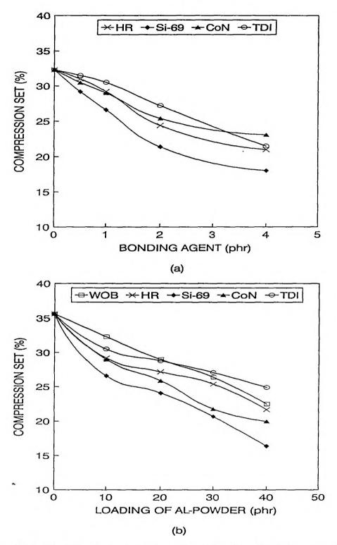
Figure III.8. Variation in compression set as a function of (a) the amount of bonding agents on natural rubber-aluminium powder (10 phr) composites and (b) the amount of aluminium powder in NR
