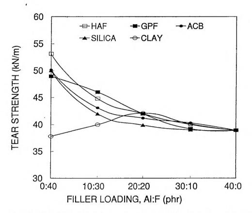
Figure V.5. Variation of tear strength with aluminium powder in presence of various fillers
