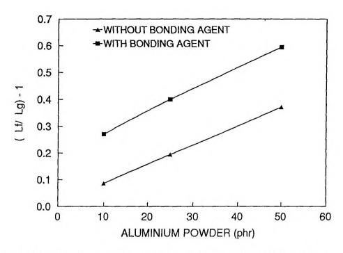
Figure IV.2. Westlinning plots of rheometric data. Effect of aluminium Powder with and without bonding agent
