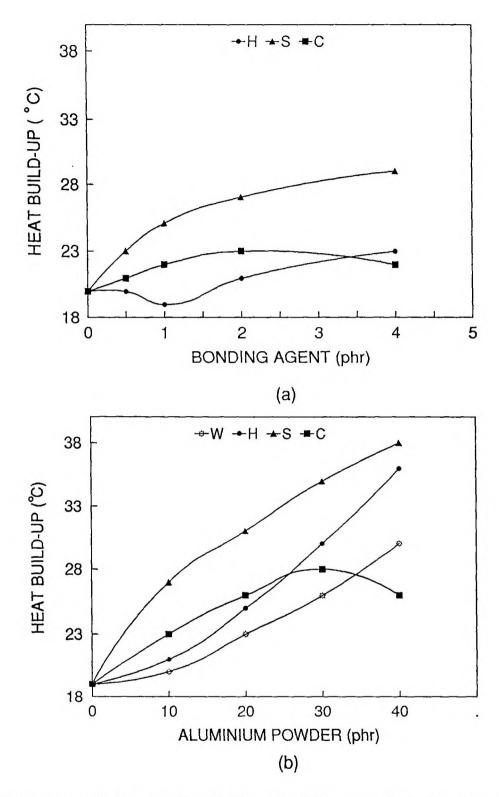
Figure XI.11. Variation of heat build-up in SBR composites as a function of (a) the amount of bonding agent at 10 phr of aluminium powder (b) the amount of aluminium powder
