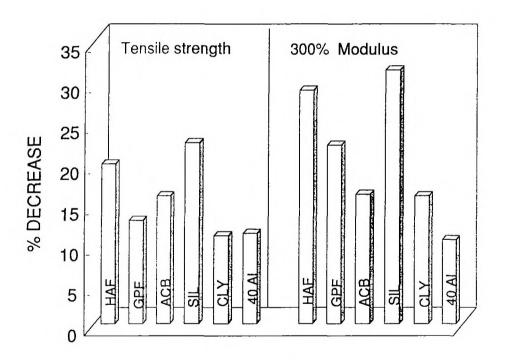
Figure VIII.1. Percentage decrease in tensile strength and modulus (300%) of NR vulcanizates containing various fillers, after ageing at 70°C for 14 days
