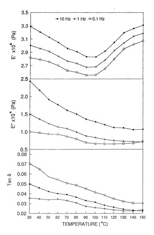
Figure VII.13. Frequency dependence of E', E" and  $tan\delta$  for natural rubber composites containing 30 phr aluminium powder
