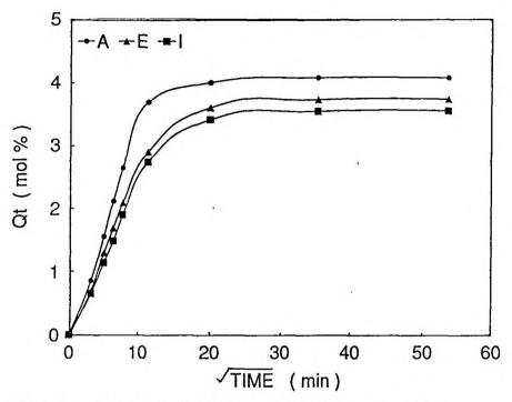
Figure IV.3a. Sorption curves for DCP system in toluene at 27°C
