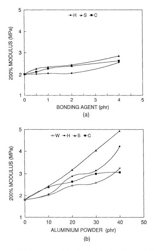
Figure XI.3. Variation of 200% modulus in SBR composites as a function of (a) the amount of bonding agent at 10 phr of aluminium powder (b) the amount of aluminium powder
