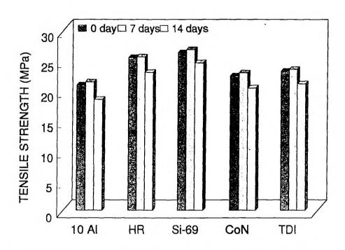
Figure VIII.4. Dependence of tensile strength with ageing at 70°C for NR-aluminium powder (10 Phr) composites containing different bonding agents
