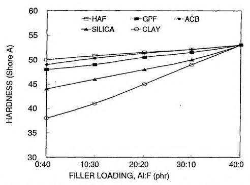
Figure V.3. Variation of hardness with aluminium powder in presence of various fillers
