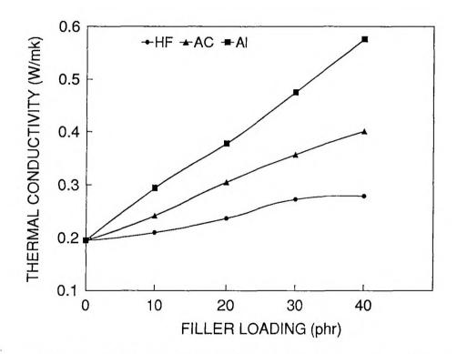
Figure X.7. Thermal conductivity of SBR composites with different fillers
