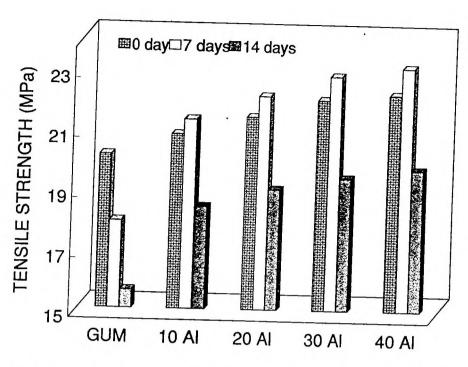
Figure VIII.2. Variation in tensile strength of aluminium powder filled natural rubber composites after ageing at 70°C
