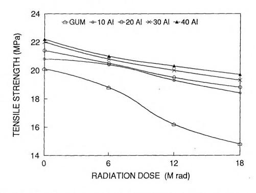
Figure VIII.7. Effect of gamma radiation on natural rubber-aluminium Powder Composites
