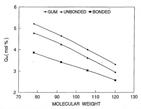
Figure IV.6a. Dependence of maximum mol% uptake on molecular weight of solvent on CV system for aromatic solvents
