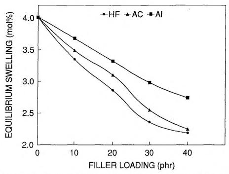
Figure X.5. Equilibrium swelling values of SBR composites with different fillers (swelling solvent, toluene at 27°C)
