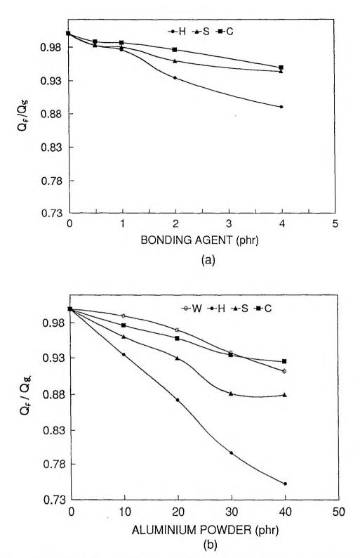
Figure XI.8. Variation of  $Q_1/Q_2$  values in SBR composites as a function of (a) the amount of bonding agent at 10 phr of aluminium powder (b) the amount of aluminium powder
