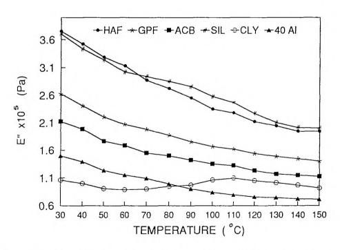
Figure VII.2. Dependence of E" with temperature of various fillers incorporated natural rubber composites at a frequency of 1.0 Hz
