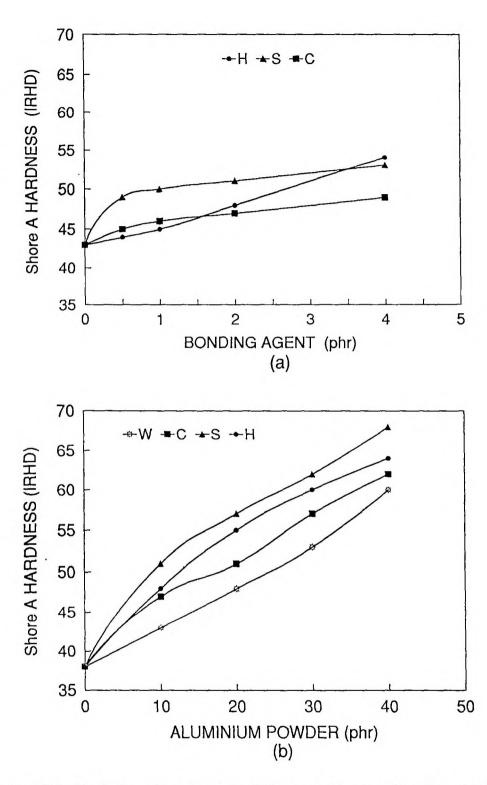
Figure XI.9. Variation of hardness in SBR composites as a function of (a) the amount of bonding agent at 10 phr of aluminium powder (b) the amount of aluminium powder
