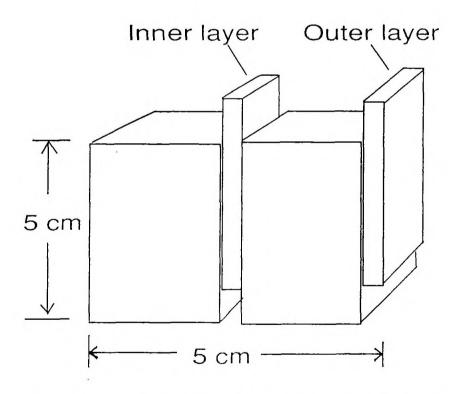
Figure IX.2. Samples from inner and outer layers of a rubber cube for swelling studies
