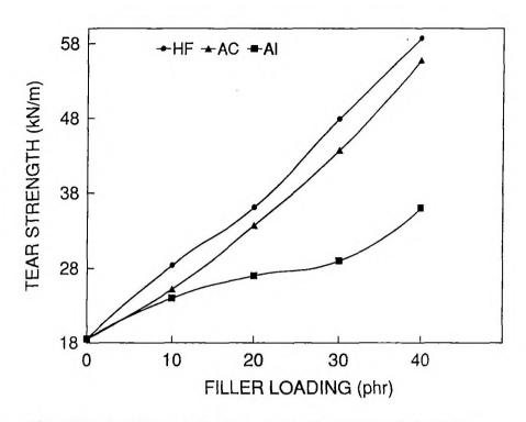
Figure X.2. Effect of filler on the tear strength of SBR vulcanizates
