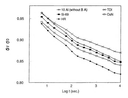
Figure VI.6. Effect of bonding agents on the stress relaxation curves of NR-aluminium powder composites (at 100% elongation)
