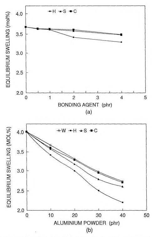
Figure XI.6. Variation of equilibrium swelling in SBR composites as a function of (a) the amount of bonding agent at 10 phr of aluminium powder (b) the amount of aluminium powder (solvent, toluene at 27°C)
