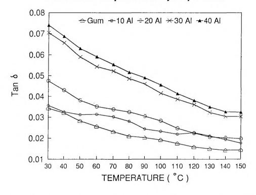
Figure VII.6. Variation of  $tan\delta$  with temperature of natural rubber composites with aluminium powder at a frequency of 10 Hz
