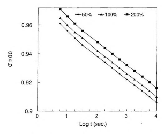
Figure V1.1. Stress relaxation curves of natural rubber (mix gum) at various strain levels
