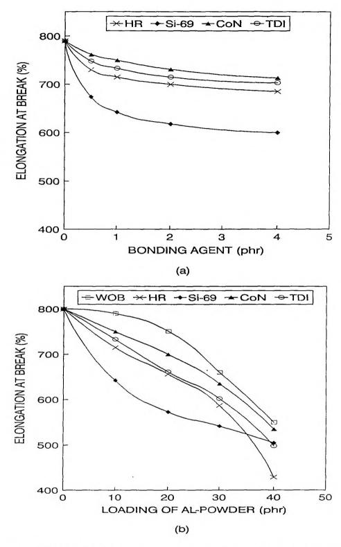
Figure III.5. Variation in elongation at break as a function of (a) the amount of bonding agents on natural rubber-aluminium powder (10 phr) composites and (b) the amout of aluminium powder in NR
