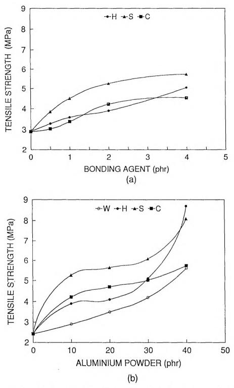
Figure XI.4. Variation of tensile strength in SBR composites as a function of (a) the amount of bonding agent at 10 phr of aluminium powder (b) the amount of aluminium powder
