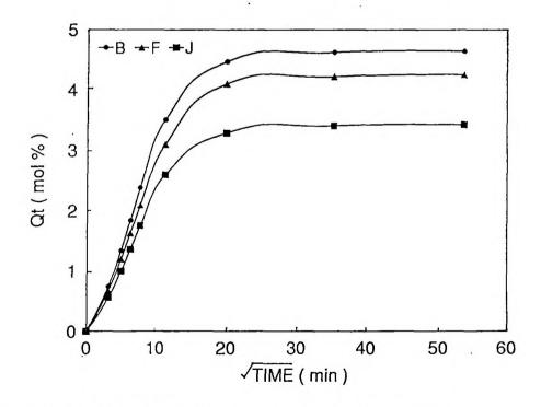
Figure IV.3b. Sorption curves for CV-system in toluene at 27°C
