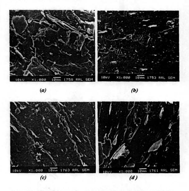
Figure XI.13. SEM photographs of tensile fractural surface of 10 phr aluminium powder filled SBR vulcanizates with and without the presence of bonding agents.
