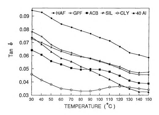
Figure VII.3. Variation of  $tan\delta$  with temperature of natural rubber with various fillers at a frequency of 10 Hz
