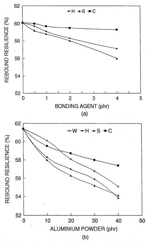
Figure XI.12. Variation of rebound resilience in SBR composites as a function of (a) the amount of bonding agent at 10 phr of aluminium powder (b) the amount of aluminium powder
