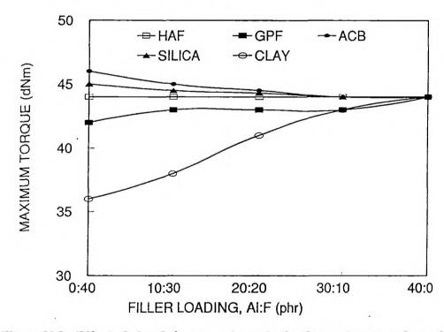
Figure V.2. Effect of aluminium powder substitution on torque values of NR-composites containing various fillers
