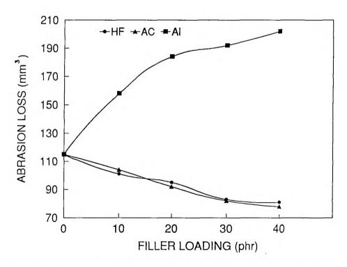
Figure X.3. Abrasion loss due to loading of HAF, acetylene black and aluminium powder on SBR
