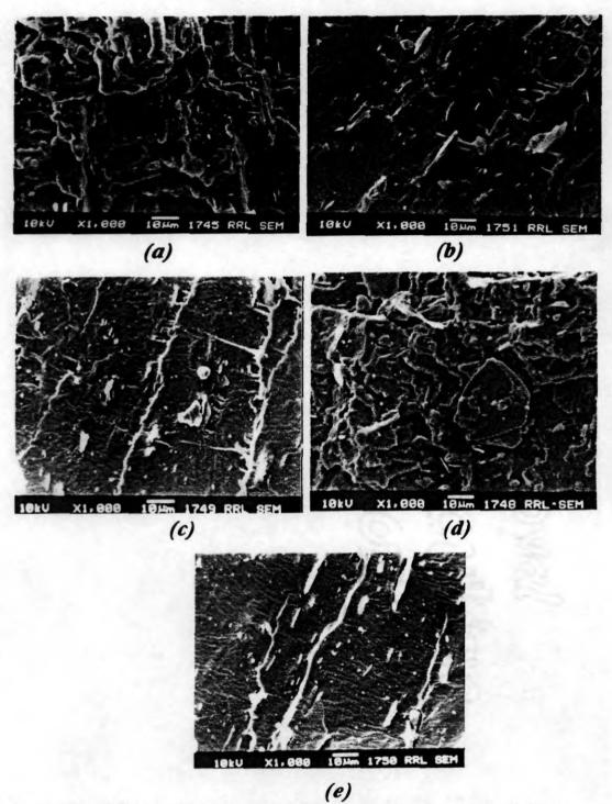
Figure VI.7. SEM photographs of tensile fractured surface of aluminium powder filled (10 phr) natural rubber composites (magnification, x 1000) (a) without bonding agent (b) with HR syste (c) with Si-69 (d) with CoN (e) with TDI
