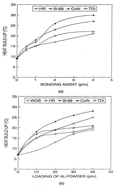
Figure III.6. Variation in heat build-up as a function of (a) the amount of Bonding agents on natural rubber - aluminium powder (10 phr) composites and (b) the amount of aluminium powder in NR
