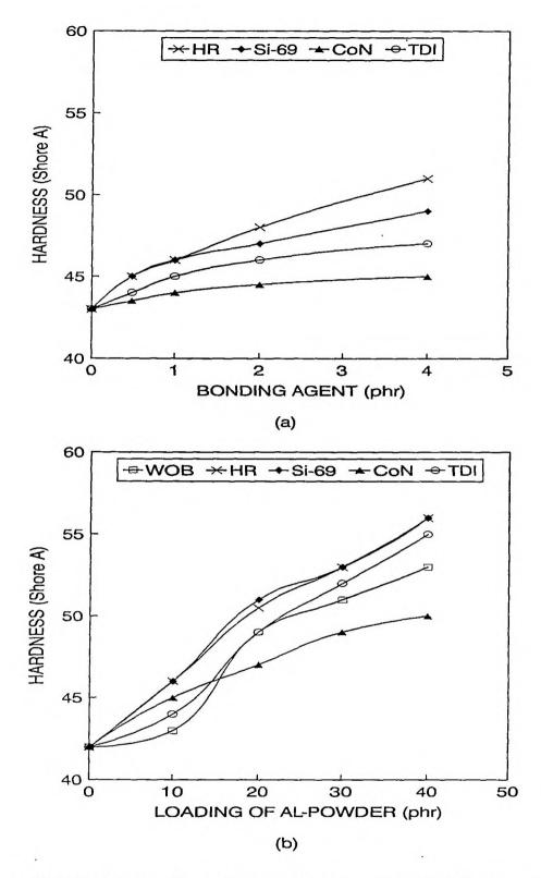
Figure III.1. Variation in Shore A hardness as a function of (a) the amount of bonding agents on natural rubber-aluminium powder (10 phr) composites and (b) the amount of aluminium powder in NR
