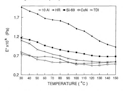
Figure VII.11. Dependence of E" with temperature of NR-aluminium powder filled composites with various bonding agents at a frequency of 1.0 Hz
