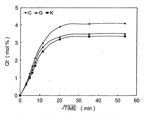
Figure IV.3c. Sorption curves for EV-system in toluene at 27°C
