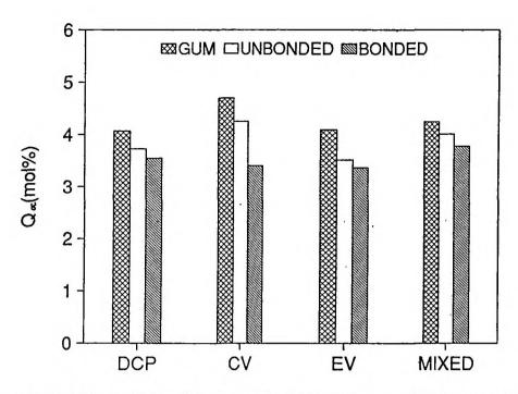
Figure IV.4. Effect of aluminium powder (10 phr) on equilibrium swelling of NR vulcanizates with and without bonding agents (solvent – toluene at 27°C)
