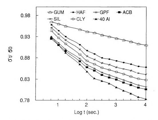
Figure V1.3. Stress relaxation curves of natural rubber composites with various fillers (at 100% elongation)
