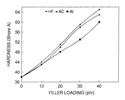
Figure X.1. Variation in hardness with filler loading in SBR-vulcanizates
