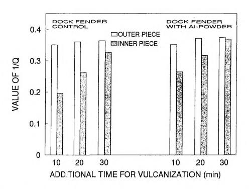
Figure IX.3. 1/Q values of inner and outer pieces of 5 cm cube of dock fender compound with and without aluminium powder
