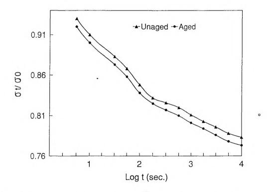
Figure V1.5. Stress relaxation curves of natural rubber composites containing 40 phr aluminium powder (after ageing, at 100% elongation)
