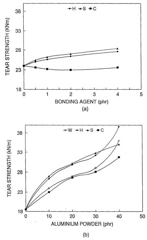
Figure XI.10. Variation of tear strength in SBR composites as a function of (a) the amount of bonding agent at 10 phr of aluminium powder (b) the amount of aluminium powder
