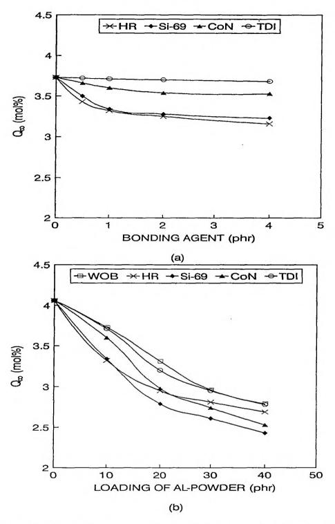
Figure III.11. Variation in equilibrium swelling as a function of (a) the amount of bonding agents on natural rubber – aluminium powder (10 phr) composites and (b) the amount of aluminium powder in NR [solvent – Toluene at 27°C]
