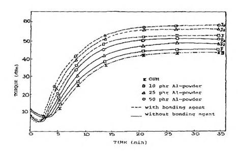
Figure IV.1. Rheometric data of aluminium powder loaded natural rubber composites containing conventional vulcanizing systems.
