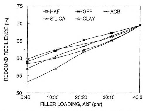
Figure V.4. Variation of resilience with aluminium powder in presence of various fillers
