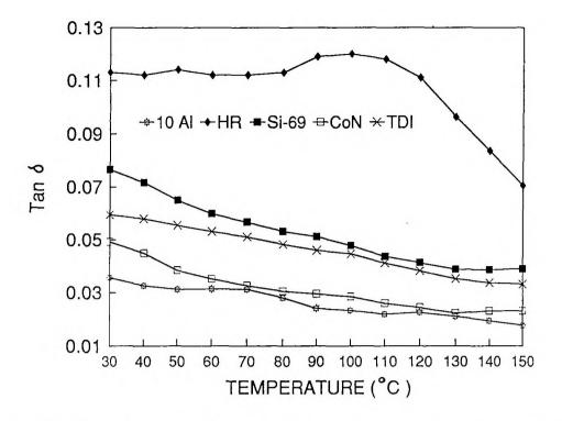
Figure VII.12. Variation of tan  $\delta$  with temperature of NR-aluminium powder composites with various bonding agents at a frequency of 10 Hz
