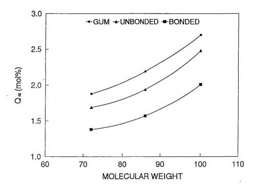
Figure IV.6b. Dependence of maximum mol% uptake on molecular weight on CV system for aliphatic solvents
