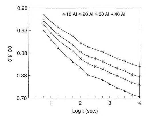
Figure V1.4. Stress relaxation curves of natural rubber composites containing aluminium powder (at 100% elongation)
