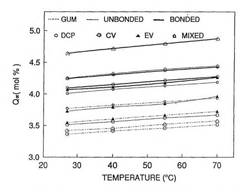
Figure IV.7. Dependence of temperature on the maximum uptake of toluene
