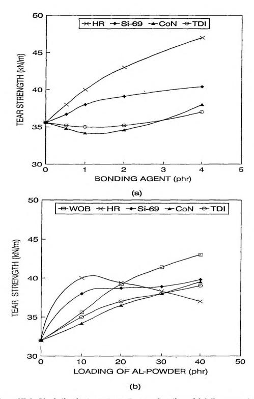
Figure III.9. Variation in tear strength as a function of (a) the amount of bonding agents on natural rubber aluminium powder(10 phr) composites and (b) the amount of aluminium powder in NR
