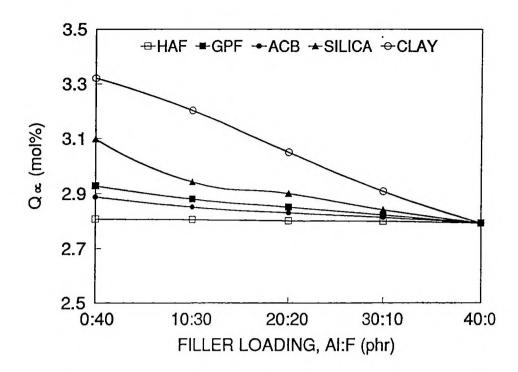
Figure V.9. Variation of equilibrium-swelling with aluminium powder in presence of various fillers (swelling in toluene at 27°C)
