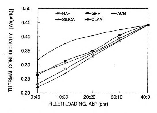
Figure V.10. Variation of thermal conductivity with aluminium powder in presence of various fillers
