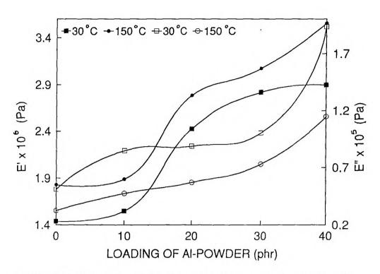
Figure VII.7. Variation of E' with loading of aluminium powder in natural rubber at different temperatures at 0.1 Hz
