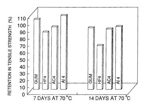
Figure X.6. Percentage retention in tensile strength after ageing at 70°C
