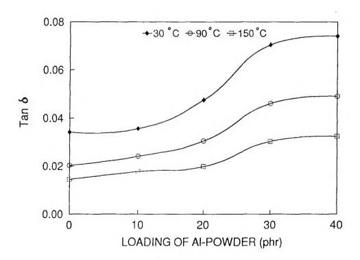
Figure VII.8. Variation of  $tan\delta$  with loading of aluminium powder in natural rubber at different temperatures at a frequency of 10 Hz
