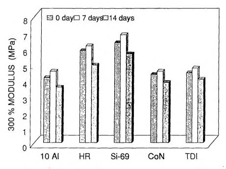
Figure VIII.5. Dependence of 300% modulus with ageing at 70°C for NR-aluminium powder (10 Phr) composites containing different bonding agents
