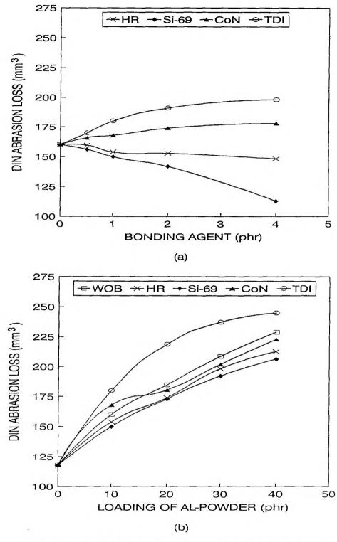
Figure III.7. Variation in DIN abrasion loss as a function of (a) the amount of bonding agents on natural rubber-aluminium powder (10 phr) composites and (b) the amount of aluminium powder in NR
