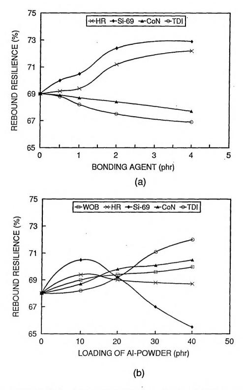
Figure III.2. Variation in rebound resilience as a function of (a) the amount of bonding agents on natural rubber - aluminium powder (10 phr) composites and (b) the amount of aluminium powder in NR
