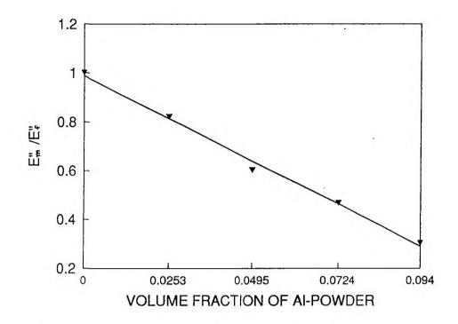
Figure VII.14. E."/E." as a function of aluminium powder concentration at 35°C, 10 Hz
