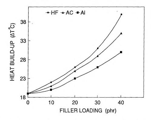
Figure X.4. Heat build-up values of SBR-vulcanizates containing HAF, acetylene black and aluminium powder
