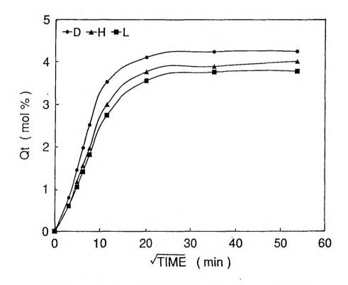
Figure IV.3d. Sorption curves for mixed system in toluene at 27°C
