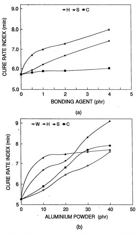
Figure XI.2. Variation of cure rate index in SBR composites as a function of
