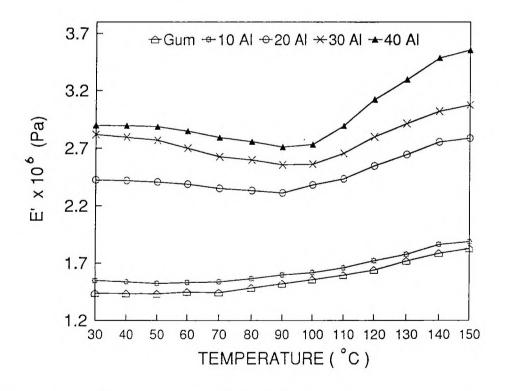
Figure VII.4. Variation E' with temperature of natural rubber composites with aluminium powder at a frequency of 0.1 Hz
