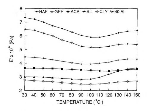
Figure VII.1. Variation E' with temperature of natural rubber composites with various fillers at a frequency of 1.0 Hz
