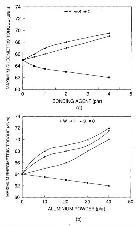
Figure XI.1. Variation of maximum rheometric torque in SBR composites as a function of (a) the amount of bonding agent at 10 phr of aluminium powder (b) the amount of aluminium powder
