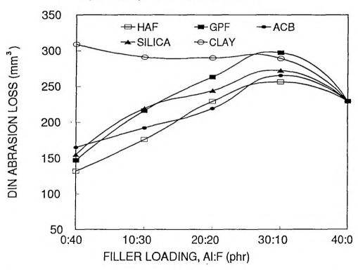
Figure V.7. Dependence of abrasion loss with aluminium powder on various filler incorporated NR-composites
