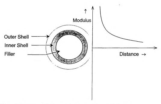
Figure VII.9. Schematic representation of rubber shell model
