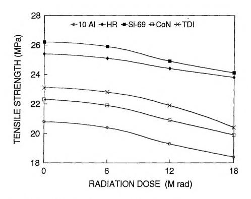
Figure VIII.8. Variation in tensile strength with gamma irradiation for NR-aluminium powder (10Phr) composites containing different bonding agents
