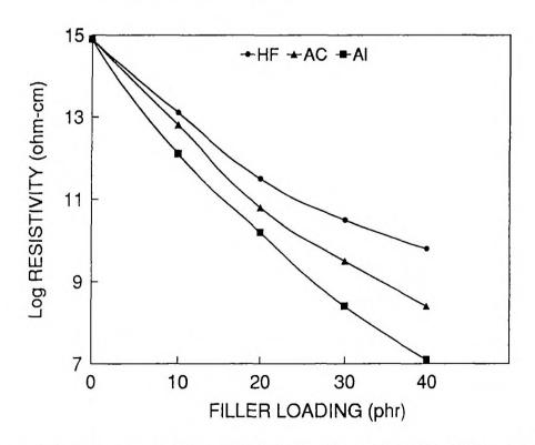
Figure X.9. Volume resistivity of SBR composites with HAF, acetylene black and aluminium powder fillers
