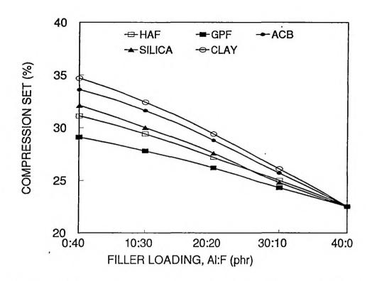
Figure V.8. Dependence of compression set with aluminium powder on various filler incorporated NR-composites
