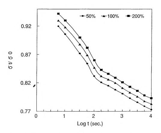
Figure VI.2. Stress relaxation curves of 40 phr aluminium powder filled NR composites at various strain levels
