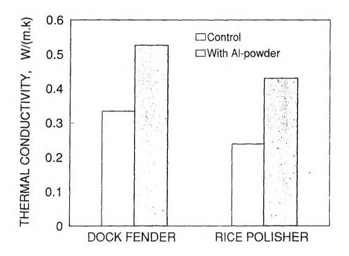
Figure IX.1. Thermal conductivity increase of the composites by the replacement of 20 phr HAF with Aluminium powder
