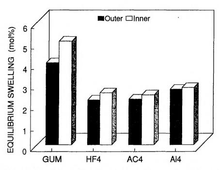
Figure X.8. Equilibrium swelling  $(Q\alpha)$  values of inner and outer layers of 25.4 mm cube of SBR compounds, vulcanized for additional 5 min over optimum cure time
